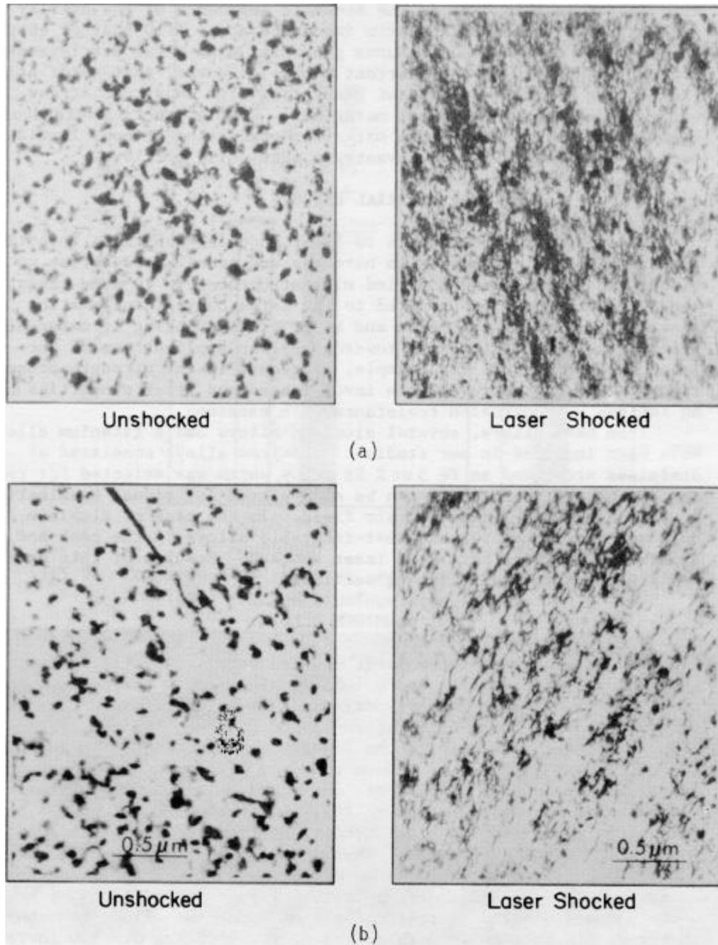
Fig. 4. Microstructures of unshocked and shocked aluminum alloys.
