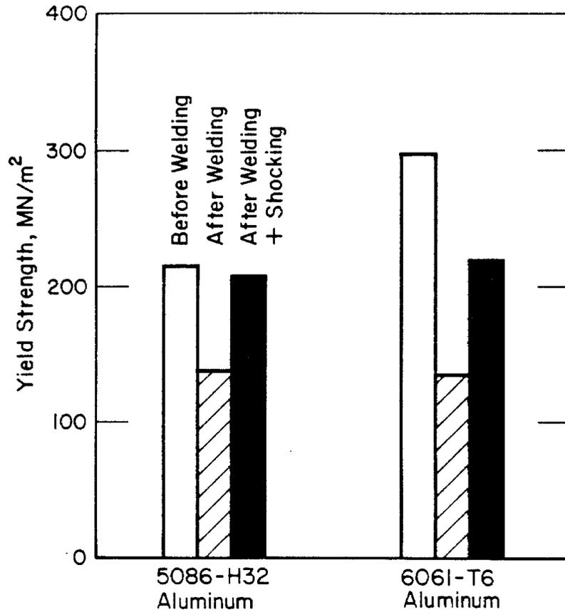
Fig. 5. Comparison of the 0.2% offset yield strength of welded and laser shocked aluminum alloys.
