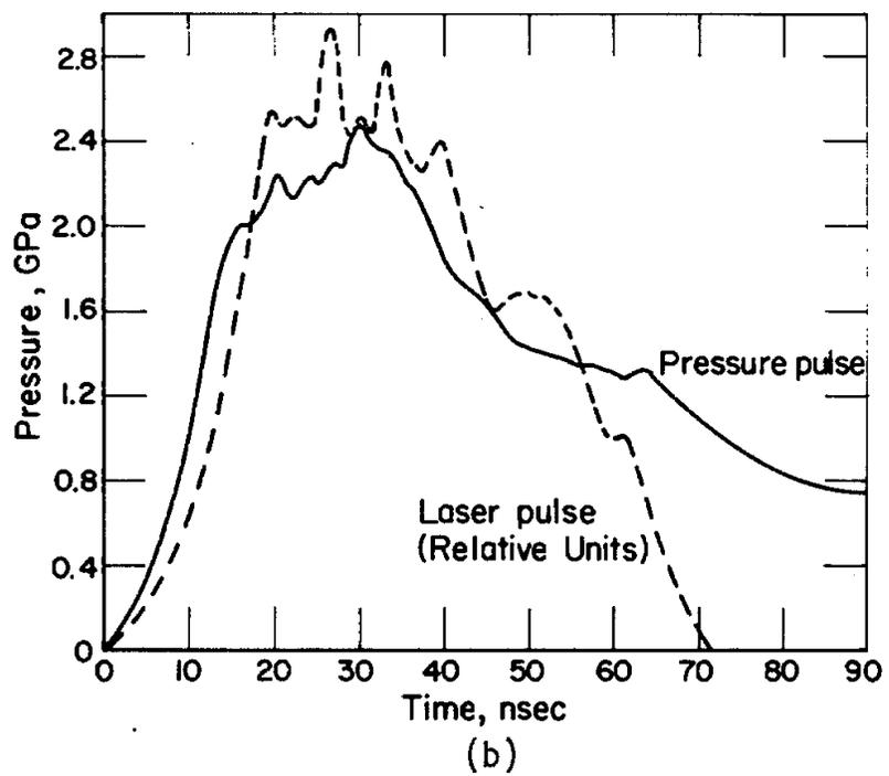
Fig. 2. Comparison of measured laser pulses with pressure pulses. (a) Quartz overlay. (b) Water overlay.
