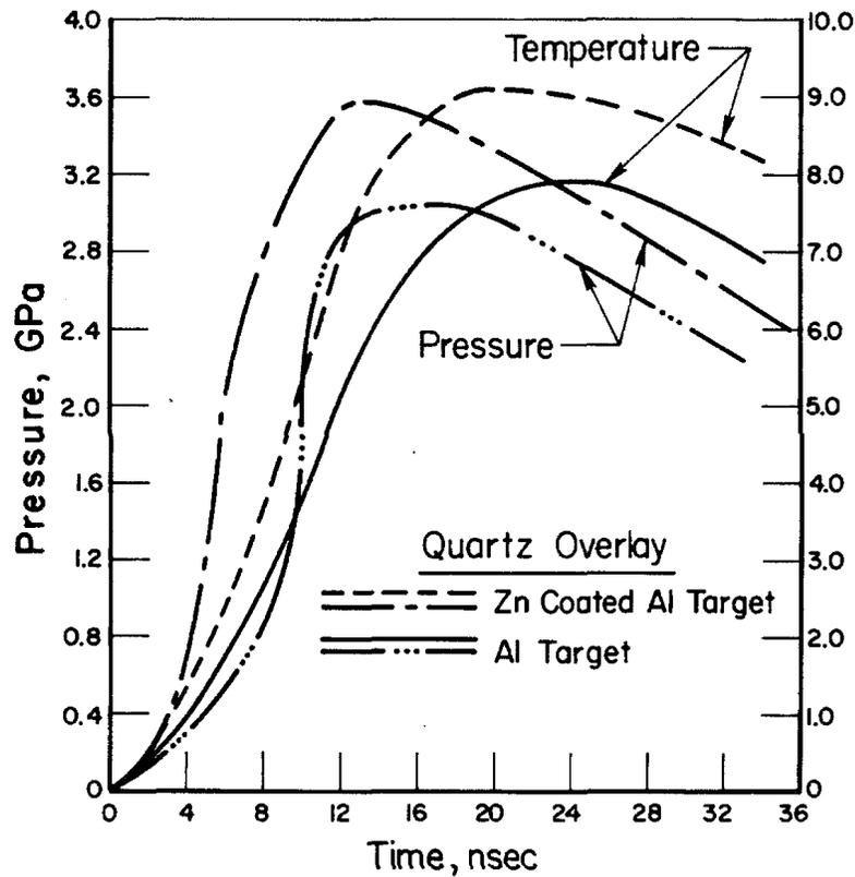
Fig. 3. Comparison of temperature and pressure histories for an aluminum and zinc target.
