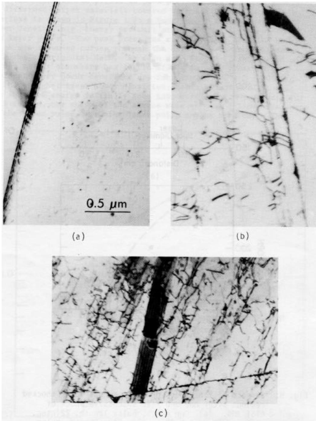
Fig. 9. Effect of multiple shocks on dislocation substructure in 304 stainless steel. The shocking conditions were black paint plus water overlay, 4.9 GPa peak pressure and a 22 nsec pulse duration. The specimens were shocked from one side only. (a) Unshocked. (b) One shock. (c) Five shocks.
