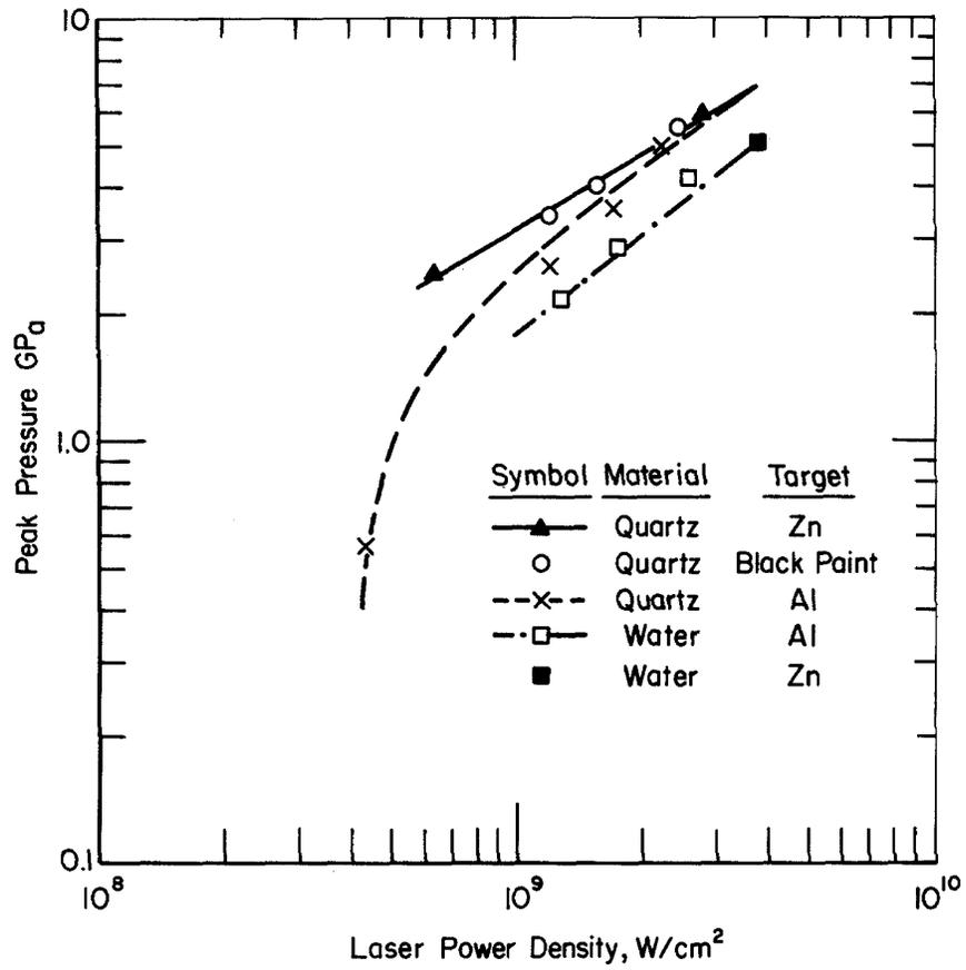
Fig. 1. Comparison of predicted and measured peak pressures generated in different target films confined by quartz or water overlays.
