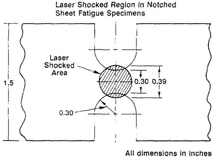
Figure 8. Specimen and Laser Shocking Configuration for the Thin, AISI 4340 Steel Sheet. The Dimensions are in Inches
