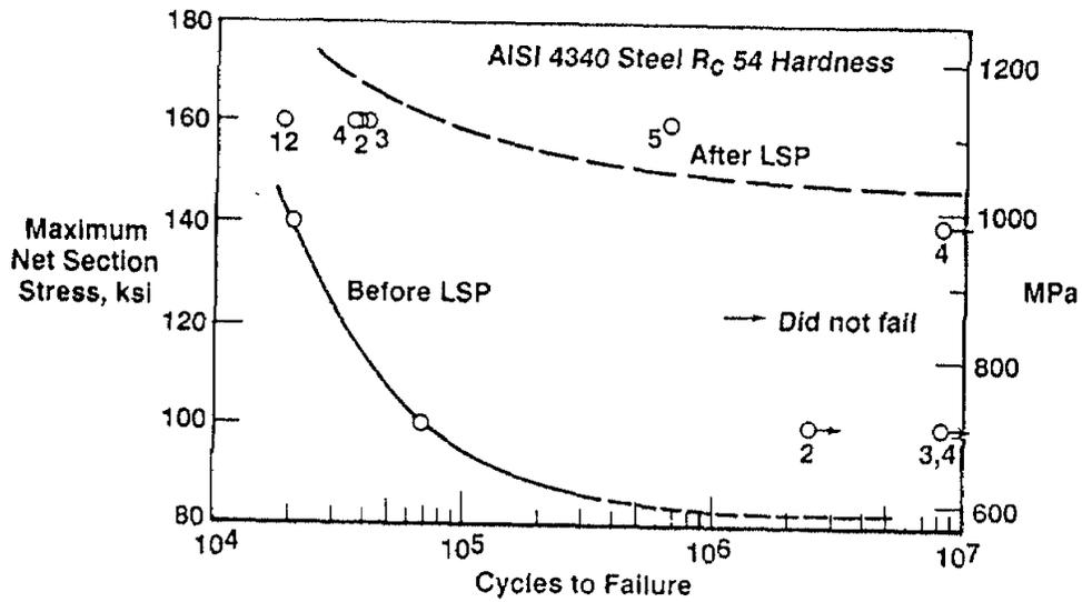
Figure 9. Fatigue of Shocked and Unshocked AISI 4340 Steel Sheet Heat Treated to  $R_c$  54. Tested at a Stress Ratio of 0.1
