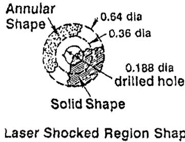
Figure 5. Specimen Configuration and Laser Shocking Arrangement for Tensile Fatigue Specimens Containing a Hole. The Dimensions are in Inches
