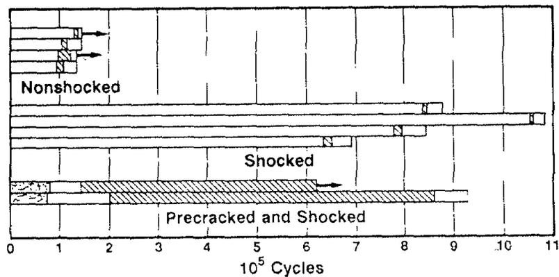
Represent the Cycles to Grow the Crack from 6 to 11 mm Long.
