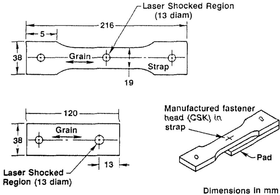
Figure 3. Specimen Configuration for the Fastened, Fretting Fatigue Specimen. All Dimensions are in Millimeters
