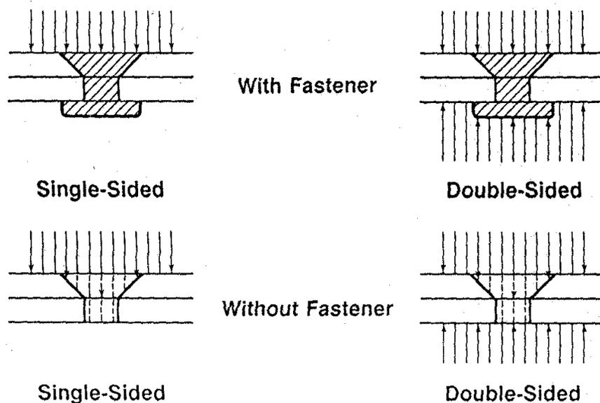
Figure 10: Possible Configurations for Laser Shock Processing of Fastener Holes
