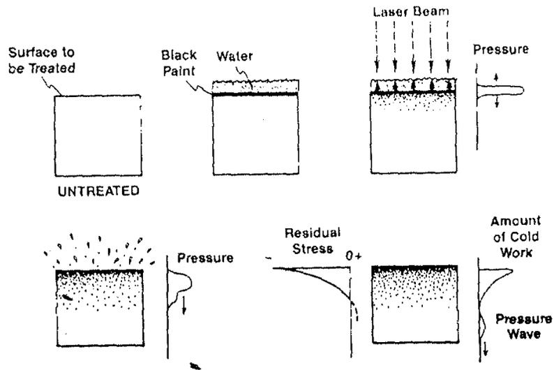
Figure 1. Schematic of the Laser Shocking Process, Showing the Overlays and the Action of the Pressure and Associated Stress Wave to Produce a Surface Residual Compressive Stress
