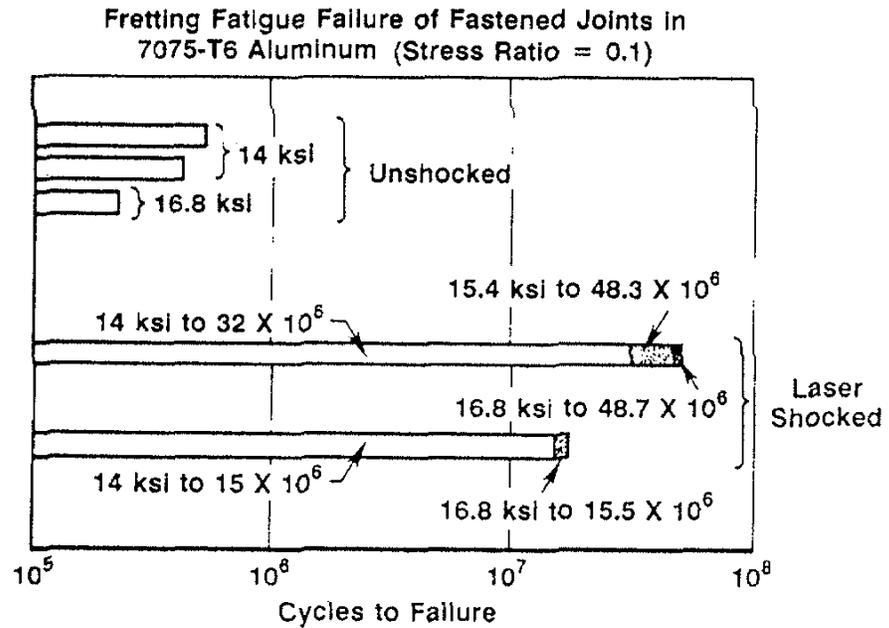
Figure 4. Fretting Fatigue Lives of Laser Shocked and Unshocked Specimens of 7075-T6 Aluminum Tested at a Stress Ratio of 0.1
